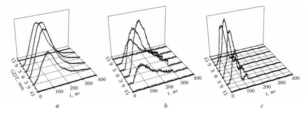
**Fig. 3.** Variability of generation pulse shape depending on the diameter of the discharge channel: total generation pulse (*a*); 3-µm pulse (*b*), 1-µm pulse (*c*).
