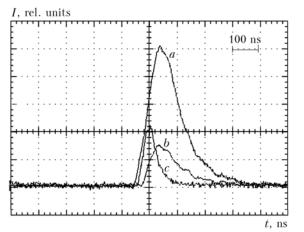
**Fig. 2.** The shape of strontium-vapor laser generation pulse: a is the total pulse; b is a 3 µm pulse, c is a 1 µm pulse.
