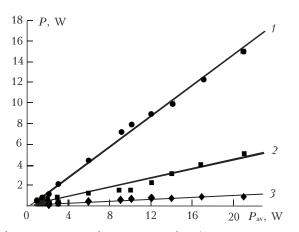
**Fig. 4.** Average radiation power distribution over spectral lines in the master oscillator-power amplifier system: generation power at 6.456  $\mu$ m line (1); total generation power at 3 (2) and at 1  $\mu$ m (3).
