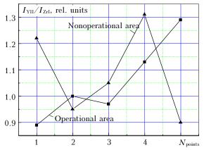
**Fig. 6.** The relation of YII ions radiation intensity at  $\lambda = 4374.9$  Å to the intensity of Zr atoms glow at  $\lambda = 4710.1$  Å. The material operational area was used in an installation designed for thin films saturation.
