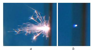
Fig. 4. Plasma glow on the surface of titanium nitrate coating (a) and substrate material 12X18H10T (b).
