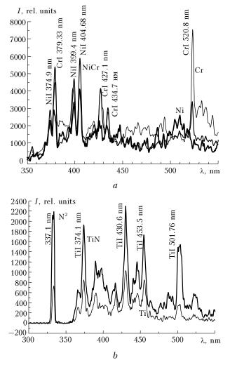
**Fig. 3.** Laser plasma glow spectrum on the surface of NiCr alloy and pure elements Ni, Cr, Ti (a) and on the surface of TiN (b) coating.
