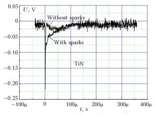
Fig. 5. The change of plasma glow (see Fig. 4) intensity with time in the presence and in the absence of sparks.
