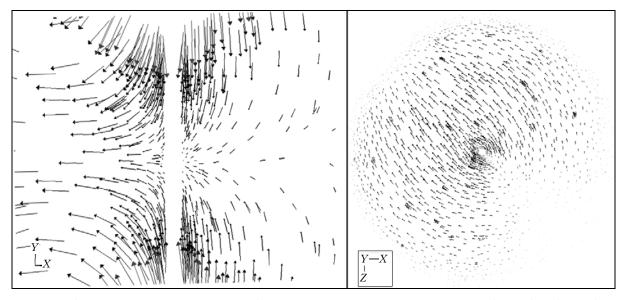
**Fig. 3.** The field of the gas motion velocity, caused by thermal slip on nonhomogeneously heated thread holders and on the thread itself. To the left, the velocity field plane passes through the holders (they are inside the visual zone); to the right, the velocity field plane is perpendicular to the thread at its middle point.
