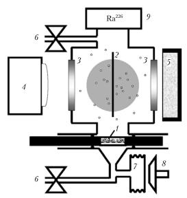
Fig. 1. Schematic view of the experimental setup: particles on nylon net before injection into cell (1); heated thread (2); four windows (3); one of two digital video-cameras (4); background illumination (5); tubes with valves for inlet and outlet of the working gas (6); membrane (7); percussive mechanism for injecting particles (8); source of gas ionization (9).
