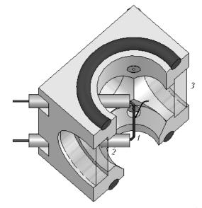
**Fig. 2.** Vertical section of the measurement cell for studying thermophoresis under microgravity conditions: heated thread (1); ceramic holders (2); window (3).
