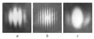
**Fig. 4.** Speckle interference patterns characterizing transversal displacement of a scatterer, when at the stage of recording the speckle interference pattern with a positive lens with f = 220 mm the matte screen was illuminated by radiation: with a plane wave (*a*); with a spherical divergent wave (*b*); with a spherical convergent wave (*c*).
