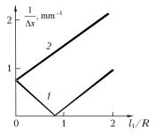
**Fig. 3.** Frequency of speckle interference fringes as a function of the curvature radius of a divergent spherical wavefront (1) and a convergent wavefront (2) for the case of a positive lens with f = 170 mm.
