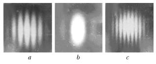
**Fig. 5.** Speckle interference patterns characterizing transversal displacement of the scatterer when the matter screen is illuminated by radiation with a plane wave (a); by a spherical divergent wave (b); by a spherical convergent wave (c).
