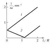
**Fig. 2.** Frequency of speckle interference fringes as a function of the curvature radius of a divergent spherical wavefront (1); of a convergent wavefront (2), for the case of a positive lens with f = 220 mm.
