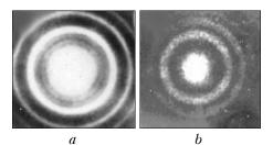
Fig. 8. Distribution of illumination in reconstruction of a multi-exposure specklogram: in the plane of the interference pattern localization (a), beyond the localization plane (b).
