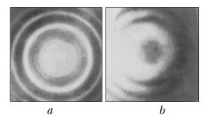
Fig. 9. Speckle interference patterns demonstrating the parallax of interference fringes in non-shifted (a) and shifted (b) positions of the specklogram at the stage of its reconstruction.
