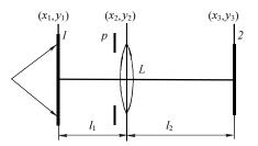
**Fig. 1.** Schematic of double-exposure specklogram recording: matte screen 1; photographic plate 2; positive lens L; aperture diaphragm p.
