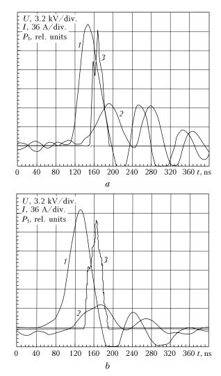
**Fig. 4.** Oscillogramms of voltage (1), current (2), and lasing (3) for the voltage doubling circuit with MPC: GDT1 (*a*) and GDT2 (*b*).
