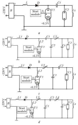
**Fig. 2.** CuBr+Ne+HBr laser pumping circuits: direct discharge circuit of the storage capacitor (*a*); circuit with magnetic pulse compression without voltage doubling (*b*)<sup>13</sup>; Blumlein voltage doubling circuit (c)<sup>5,13</sup>; voltage doubling circuit with magnetic pulse compression (*d*).<sup>2</sup>
