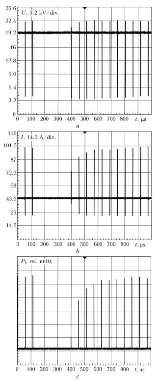
**Fig. 5.** Oscillograms of voltage (a), current (b), and lasing pulses (c) at the train operation mode with the 17.5-kHz pulse frequency in a train.
