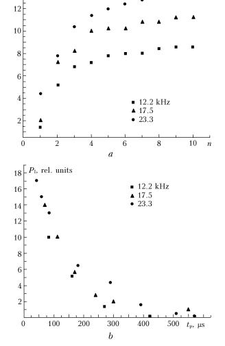
**Fig. 6.** Peak lasing power  $P_1$  as a function of pulse number in a train (*a*) and the peak lasing power in the first pulse in a train  $P_{11}$  as a function of inter-pulse pause accumulating  $t_p(b)$ .
