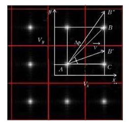
**Fig. 3.** Hartmanogram fragment:  $V_x$ ,  $V_y$  are the wind velocity projections.
