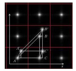
**Fig. 4.** Hartmanogram fragment:  $V_x = AC$ ,  $V_y = BC$  and  $V'_x = A'C'$ ,  $V'_y = B'C'$  are the velocity projections at the time moments  $t_1$  and  $t_2$ .
