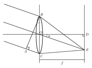
Fig. 2. Schematic of optical beam refraction by a single microlens.
