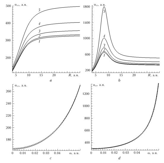
**Fig. 4.** Polarizability functions of Li<sub>2</sub> molecule:  $\alpha_{xx}(R, \omega)(a)$ ;  $\alpha_{zz}(R, \omega)(b)(\omega = 0(1), 0.01(2), 0.02(3), 0.03(4)$ , and 0.04 a.u. (5));  $\alpha_{xx}(R_{e}, \omega)(c)$ ; and  $\alpha_{zz}(R_{e}, \omega)(d)$  (solid lines – this work, dashed lines – *ab initio* calculations<sup>29</sup>).
