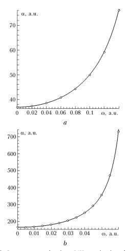
**Fig. 2.** Components of the LiH molecule dynamic polarizability tensor: polarizability function  $\alpha_{ii}(0, \omega)$  (solid line) and *ab initio* calculated polarizability of the ground state of Be atom<sup>20</sup> (circles) (*a*);  $\alpha_{ii}(\infty, \omega)$  (solid line) and sum of polarizabilities of the ground states of Li [Ref. 21] and H [Ref. 22] atoms (circles) (*b*).
