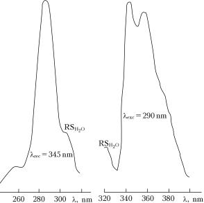
**Fig. 2.** Spectra of excitation and UV fluorescence in part *a* of the centrifuged seawater sample collected from a depth of 20 m ( $RS_{H_{2O}}$  is the Raman scattering of water).
