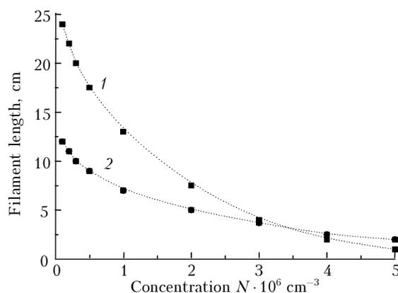
Fig. 5. Length of the filamentation zone of the laser beam as a function of the aerosol particle number concentration: (curves) calculation from the data on energy extinction<sup>8</sup> and curves 1-4 in Fig. 4 at the pulse energy  $E = 15$  mJ;  $F = 130$  cm (1) and 86 cm (2).
