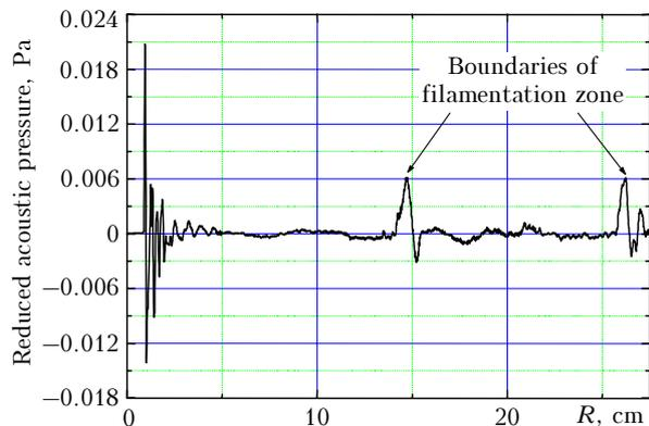
**Fig. 2.** Time scan of the acoustic signal generated by a laser beam and measured in the longitudinal direction. The acoustic pressure is reduced to a distance of 1 m:  $P_{ac,red} = P_{ac,m}R$ .
