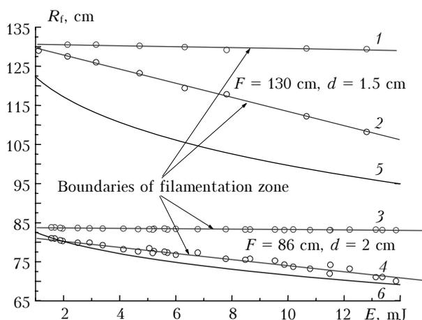
Fig. 4. Positions of the beginning (2, 4) and end (1, 3) of the filamentation zone for two focusing mirrors as functions of the input beam energy; (5, 6) theoretical dependences.
