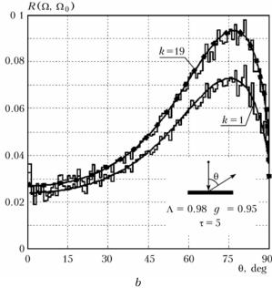
Fig. 2. The brightness coefficients of the reflected radiation: reflection from semi-infinite turbid medium (a), reflection from the layer of the optical thickness  $\tau = 5$  (b). Incidence angle is normal. Numbers denote the multiplicity of "strong" scattering k. Solid line shows the results of calculation by Eq. (15). Points indicate calculation by the modified method of spherical harmonics<sup>6</sup> and histogram shows the results of statistical simulation with the program SPIM-L.
