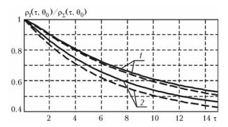
**Fig. 3.** The dependence of the ratio  $\rho_1(\tau, \theta_0)/\rho_{\Sigma}(\tau, \theta_0)$  on the optical thickness: curves (1) are for cloud cover C1, and (2) is for haze L. Incidence angle is normal. Solid line shows the results of calculations for a wavelength of 300 nm and dotted line is for a wavelength of 700 nm.
