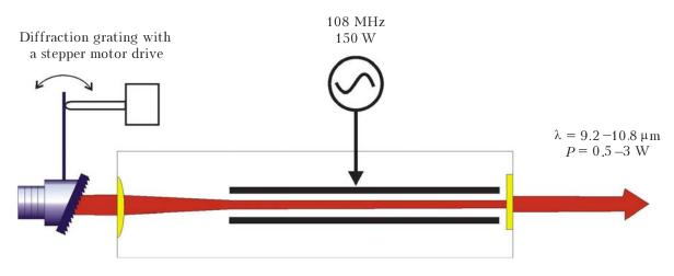
Fig. 1. Optical arrangement of a tunable waveguide CO<sub>2</sub> laser with HF excitation.
