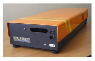
**Fig. 5.** Appearance of a laser gas analyzer with an intracavity PAD.
