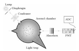
**Fig. 1.** Simplified optical scheme of photoelectric measurement of radiative flux, scattered by aerosol, with the nephelometer FAN-A.
