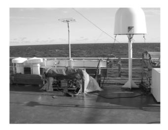
**Fig. 5.** Expedition of the Research Vessel *Professor Shtokman* in White Sea. Nephelometer was placed in a special shelter (at the center of photograph), protecting from rain, wind, and spray during storms.
