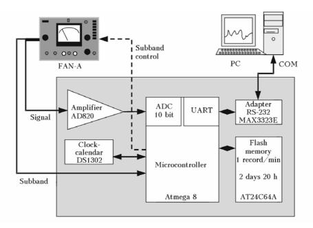
Рис. 2. Schematic view of the nephelometer microcontroller board.
