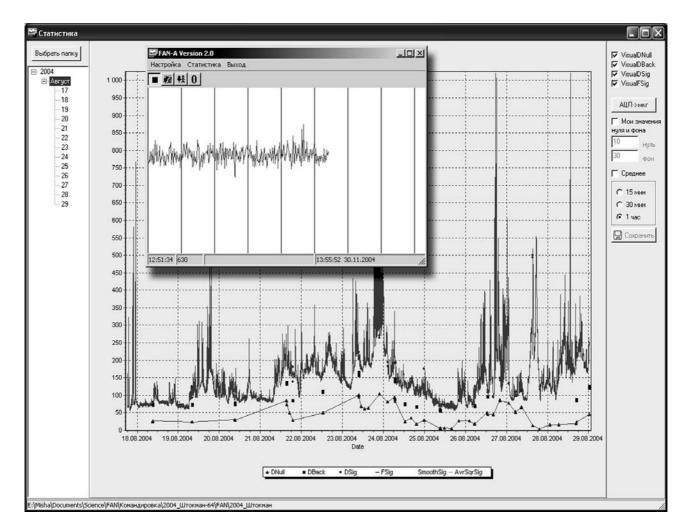
**Fig. 4.** Graphic interface of the program controlling the nephelometer controller. The controlling window with second-to second imaging of the signal is at the top to the left (the interval between vertical lines is 1 minute). The whole signal with a minute resolution is at the bottom.
