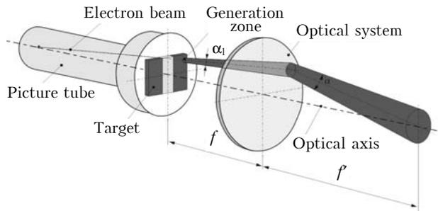
Fig. 1. Simplified optical layout of the navigation complex based on SEPSL.
