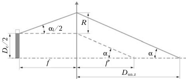
Fig. 4. Geometrical scheme of ray tracing in the scanning beam for calculating the "uncertainty zone" size.
