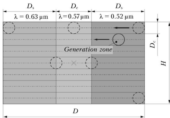
Fig. 2. Schematic view of the target used in calculating the flicker coefficient.
