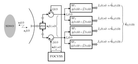
Fig. 1. Algorithm for estimation of the matrix response function of a spatially distributed non-stationary object.
