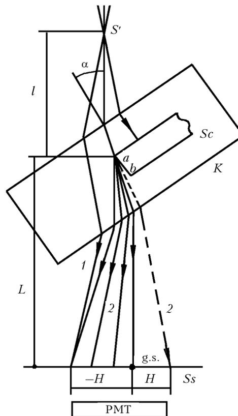
**Fig. 1.** Optical arrangement of experiments on light diffraction by a screen placed in the air or in a liquid.
