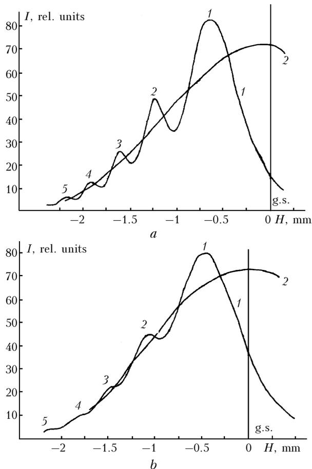
**Fig. 2.** IKS3-plate diffraction pattern when the plate is in air (*a*) and in dimethyl phthalate solution in benzyl alcohol at  $n_{\text{rel}} = 1.0054$  (*b*).
