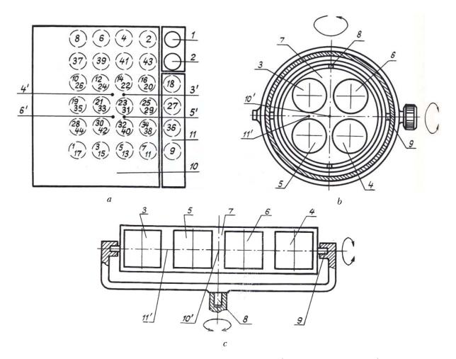
FIG. 2. The multipass four-objective matrix-array system: a) collecting mirrors; b) collecting mirrors on a circular holder; c) row variant of the arrangement of the objectives.
