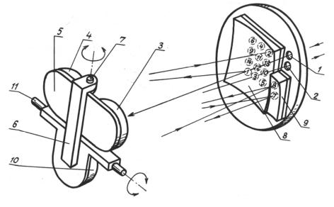
Fig. 1. Three-objective multipass matrix-array system
