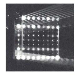
FIG. 3. Photograph of the matrix array of images on collecting mirrors after 306 passes of He-Ne laser radiation.
