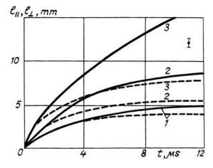
FIG. 3. The time dependence of the vertical  $l_{\parallel}$ (solid line) and horizontal  $l_{\perp}$  (broken curve) dimensions of the thermal halo of burning particles at different pressures  $P = 1.011 \cdot 10^5 Pa$  (1),  $P = 6.946 \cdot 10^4 Pa$  (2), and  $P = 4.053 \cdot 10^4 Pa$ (3).  $R = 180 \mu m$ .
