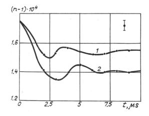
FIG. 4. Experimental dependence of the index of refraction n of the medium on the time t with pressure  $P = 6.946 \cdot 10$  Pa. Curve 1 corresponds to a particle with radius  $r_0 = 100$  µm and curve 2 corresponds to  $r_n = 250$  µm.
