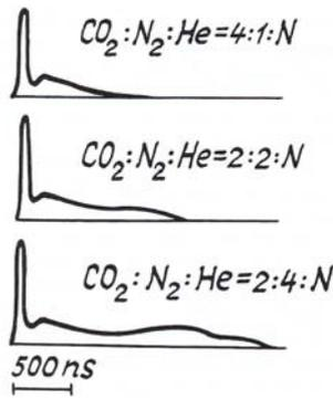
Fig. 2. Typical oscillograms of radiation for the gas mixtures  $\text{CO}_2:\text{N}_2:\text{He}$  with  $P = 0.6-1$  atm.
