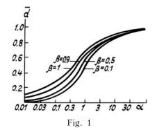
Figure 1 shows a family of curves of the normalized variances of the estimation errors  $\overline{d} = d/d_{\xi}$  as a function of the quantity  $a = d_{\xi}/d_{\eta}$  for a series of values of the parameter  $\beta$ .
