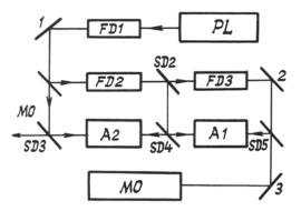
FIG. 4. Block diagram of a multifrequency laser: PL - pump laser; FD1-FD3 - frequencydoublers; 1, 2, 3 - mirrors; SD1-SD5 - spectrumdividers; A1, A2 -  $Al_2O_3$ : $Ti^{3+}$  - based amplifiers;  $MO - Al_2O_3$ : $Ti^{3+}$  - based master oscillator.
