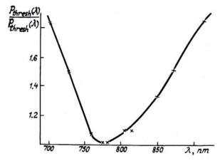
FIG. 1. The lasing threshold versus the wavelength of a  $Al_2O_3$ : $Ti^{3+}$  gased laser.
