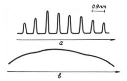
FIG. 2. Lasing spectra with Brewster (a) and normal (b) orientation of faces of the active element.
