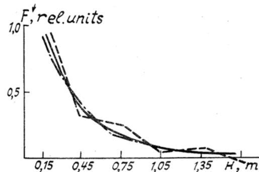
FIG. 4. Vertical profile of the incident flux in a water medium for  $\lambda = 735$  nm: the dashed curve represents the measured values; the solid curve represents the values smoothed by the Gaussian filter; the dash-dotted curve is an approximating curve.
