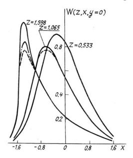
FIG. 4. Comparison of the calculations of the self-action of partially coherent radiation (solid curves) and coherent radiation: the results of Ref. 10 ( $E_r = 123$ ) and Ref. 11 ( $E_r = 246$ , dot-dashed curves.).
