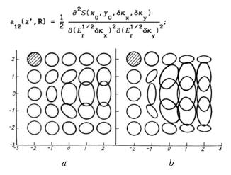
FIG. 3. Transformations of the coherence ellipse over the Gaussian beam cross-section calculated in the geometric – optics approximation at the distances z = 1 (a) and z = 1.5 (b). The cross-hatched part of the figure shows the undisturbed normalized coherence ellipse in the starting plane.
