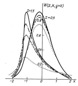
FIG. 2. The change in the profiles of the intensity of a Gaussian beam as a function of distance for the nonlinear refraction parameter  $E_r = 1$  (dotted curves),  $E_r = 4$  (dashed curves),  $E_r = 10$ (dot-dashed curves), and in the geometric – optics approximation.
