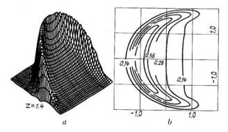
FIG. 1. The aberrational structure of a Gaussian beam obtained in the geometric optics approximation (a) and isoplets for the intensity of the same beam (b).
