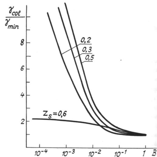
FIG. 2.  $\gamma_{\text{col}}/\gamma_{\text{min}}$  vs  $\beta$  for different normalized values of thickness  $Z_s$  of the nonlinear layer.
