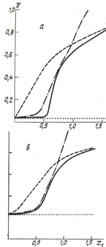
FIG. 1. The angular divergence  $\gamma$  versus the normalized values of the thickness  $z_s$  of the factor of the nonlinear layer with  $\beta = 0,001$  (a) and  $\beta = 0,05$  (b). The solid line corresponds to the optimally focused beam, the dashed line corresponds to a collimated beam, the dot-dashed line was calculated using the algorithm, and the dotted line shows the diffraction limit.
