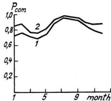
FIG. 5. Annual behaviour of communication probability with diversity reception (Tompo and Gillicule). 1 - 5 dB attenuation, 2 - 50 dB attenuation.
