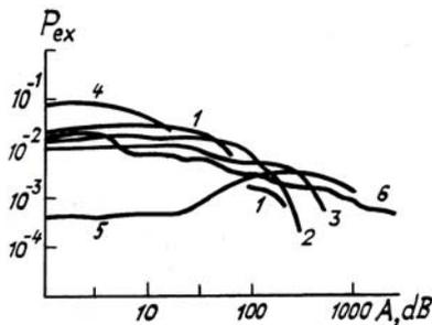
FIG. 1. Cloud attenuation probability distributions for Moscow. Summer. Numbers of curves correspond to 1 - St, 2 - Sc, 3 - As, 4 - Ci, 5 - Ns, 6 - Cu.
