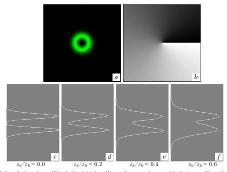
**Fig. 2.** Intensity (*a*) and the phase (*b*) of the initial collimated vortex beam with l = 1; profiles of the beam intensity calculated for some propagation distances  $z_k/z_R = 0.0$ ; 0.2; 0.4; 0.6 (*c*-*f*) using the values of the dimensionless parameter  $C_T^2 = 0.1$ .
