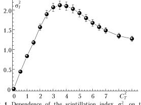
**Fig. 1.** Dependence of the scintillation index  $\sigma_I^2$  on the dimensionless turbulence parameter  $C_T^2$ , obtained in the experiment. The root-mean-square deviations shown by vertical bars are taken as the confidence intervals.
