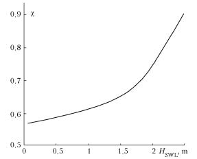
Fig. 1. Dependence of emission coefficient of soil cover on the occurrence depth of soil waters.
