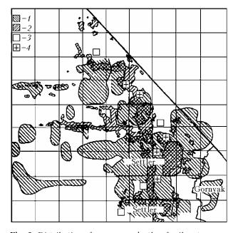
**Fig. 2.** Distribution of occurrence depths of soil waters near industrial settlers: (1) SWL < 1 m (data of aircraft microwave survey); (2) increased moisture of soil surface layer (satellite scanning); (3) boreholes with SWL > 1 m; (4) boreholes with SWL < 1 m.
