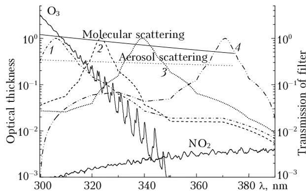
Fig. 1. Spectral dependences of optical thicknesses due to aerosol and molecular scattering, as well as O<sub>3</sub> and NO<sub>2</sub> absorption for vertical atmospheric paths of 0–100 km. Spectral transmission of filters with centers: 308 (1), 324 (2), 340 (3), and 371 nm (4).
