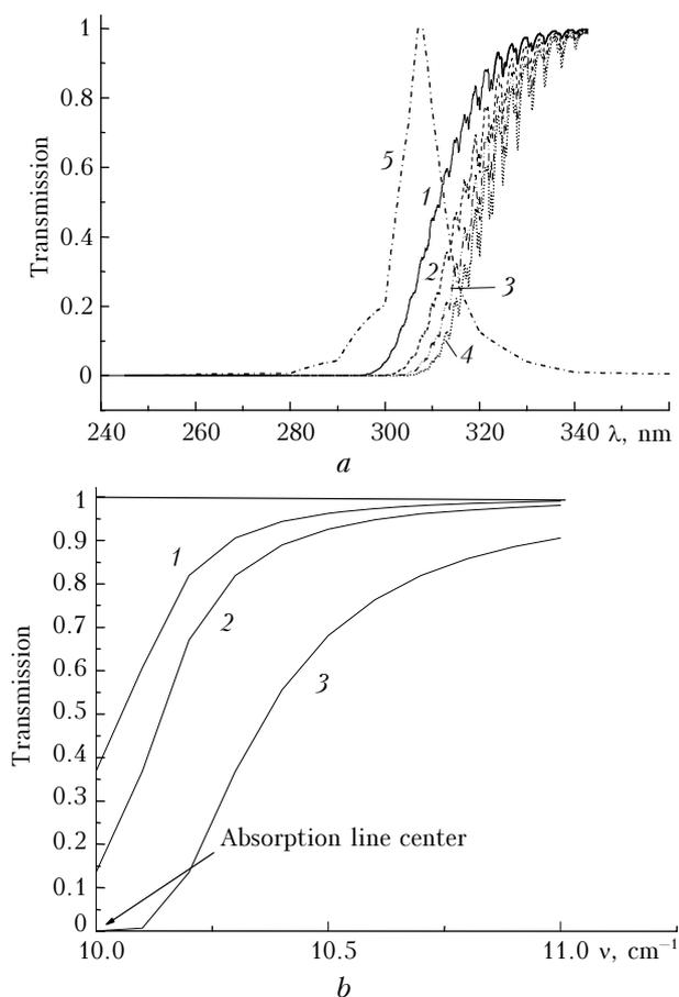
Fig. 3. Spectral transmittance of atmosphere at different air masses  $m$ : 1–4 are for  $m = 1, 2, 3, 4$ ; 5 for the spectral transmittance of the device filter for the line centered at 308 nm (a); spectral transmittance of an isolated line at different  $\tau$  values: (1 for  $\tau = 0.5$ ; 2 for 1; 3 for 3) (b).
