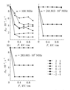
**Fig. 3.** Probabilities of the transition  $5^3D_2-2^3P_1$  as functions of the electric field frequency.
