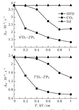
**Fig. 2.** Probabilities of transitions  $nd^3D_1-2p^3P_0$  (n = 6,7) as functions of the electric field frequency: (HFD) high-frequency discharge,  $\omega = 100$  MHz; (CO<sub>2</sub>) CO<sub>2</sub> laser,  $\omega = 241.813 \cdot 10^5$  MHz; (Nd) Nd laser,  $\omega = 283.005 \cdot 10^6$  MHz.
