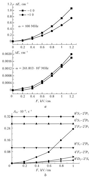
**Fig. 1.** Stark effect and transition probabilities as functions of the electric field strength for the He atom:  $8^{1}P_{1}-2^{1}S_{0}$  spectral line,  $\lambda = 329.772$  nm (*a*); probabilities of allowed and forbidden transitions (*b*).
