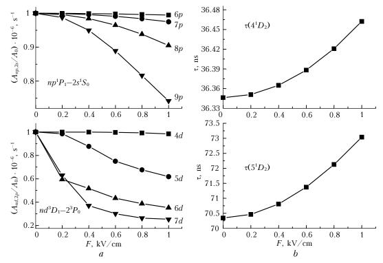
**Fig. 4.** Behavior of the transition probabilities and lifetimes of energy levels for the He atom in the high-frequency discharge: probabilities of the transitions nlJ-n'l'J(a); lifetime of the  $nd^{1}D_{2}$  states (n = 4, 5) (b).
