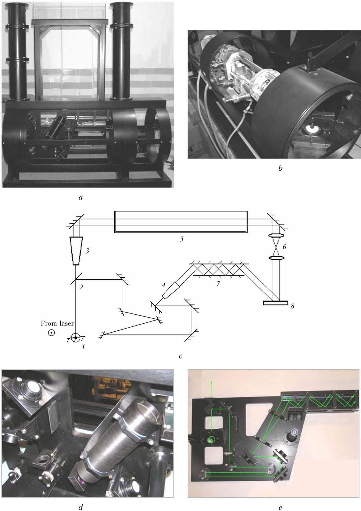
**Fig. 1.** General view of the simulator (*a, b*) and its optical arrangement (*c*); module for formation of the object beam: (*d*) as a part of the simulator; (*e*) separately from the simulator; the light line shows the beam path; (*c*) beam-turning mirror 1, beam splitter 2, collimators (Galileian telescopic system) 3 and 4, glass cell modeling the studied volume 5, optical system of image transfer (Keplerian telescopic system) 6, mirror system 7; photoplate 8.
