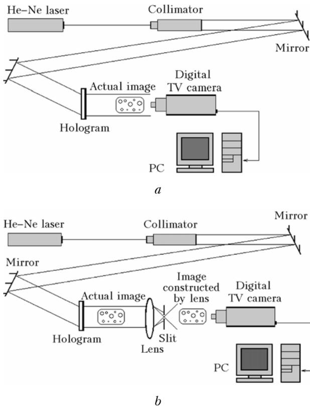
**Fig. 2.** Scheme of reconstruction of holographic images (a); scheme with filtering of spatial frequencies (b).
