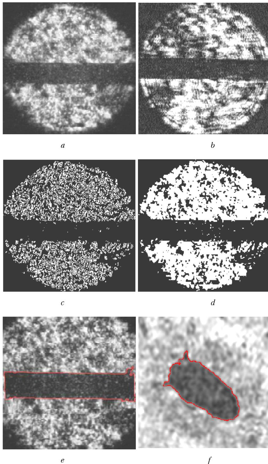
**Fig. 5.** Examples of the instrumental and numerical processing of holographic images, including the detection of boundaries: (a) initial image; (b) result of the instrumental processing using the optical set up shown in Fig. 2b; (c) numerical processing by the gradient filter; (d) numerical processing by the Sobel's filter; (e, f) results of operation of the algorithm, detecting the boundaries.
