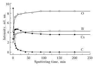
**Fig. 3.** Intensity profiles of Cs  $3d_{5/2}$ , B 1s, O 1s, and C 1s lines as functions of time of CBO surface ion sputtering.
