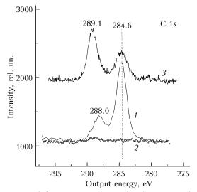
**Fig. 2.** Detailed XPS-spectrum of the C 1*s* level: *1* corresponds to polished BBO surface, *2* is to the same surface after ion sputtering during 95 min, and *3* corresponds to BaCO<sub>3</sub> powder.
