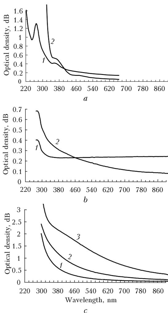
**Fig. 1.** Absorption spectra of dispersions with NPs: (a) platinum, particle size: up to 10 nm (1), up to 100 nm (2); (b) aluminum, particle size: up to 600 nm (1), from 2600 nm (2); (c) ATO, particles size: from 200 to 400 nm (1), from 200 to 400 nm (with micron-sized particles up to 2% of the mass) (2), from 400 to 1050 nm (with micron-sized particles up to 10% of the mass) (3).
