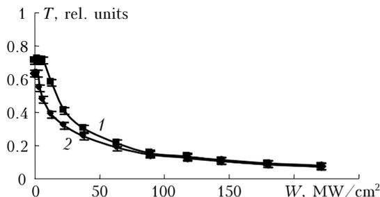
**Fig. 5.** Transmittance of the studied aluminum-based nonlinear media as a function of the excitation power density. Excitation at 532 nm, particle size: up to 600 nm (1), from 2600 nm (2).
