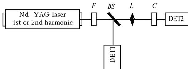
**Fig. 2.** Schematic of the experimental setup for investigation of the dependence of the medium transmittance on the power density of the exciting radiation: neutral-density filters  $F$ , beam-splitting plate  $BS$ , lens  $L$ , cell with the studied solution  $C$ , ED-100A pyroelectric detectors DET1, 2.
