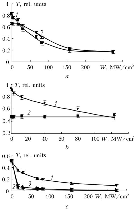
**Fig. 3.** Transmittance of the studied platinum-based nonlinear media as a function of the excitation power density: (a) excitation at 532 nm, NPs with the size up to 10 nm (1) and 100 nm (2); (b) excitation at 1064 nm, NPs with the size up to 10 nm (1) and 100 nm (2); (c) excitation at 532 nm, NPs with the size up to 10 nm (1), PC792 dye (2), and 1:1 mixture of the media 1 and 2 (3).
