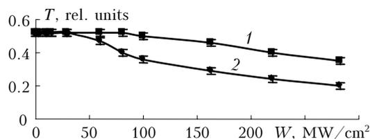
**Fig. 4.** Transmittance of the studied ATO-based nonlinear media as a function of the excitation power density. Excitation at 532 nm, particle size: from 200 to 400 nm (1); from 400 to 1050 nm (including micron-sized particles up to 10% of the mass) (2).
