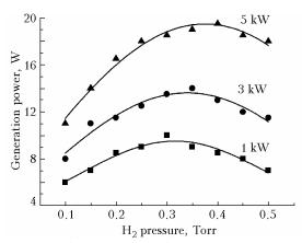
Fig. 2. Dependence of the radiation power of CuBr+Ne laser on the pressure of  $H_2$  admixture at different levels of pump power. The buffer gas, Ne, pressure is 25 Torr.
