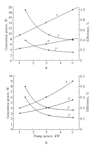
**Fig. 1.** Dependence of the radiation power (1) and the efficiency (2) of CuBr+Ne+H<sub>2</sub> laser as well as of the radiation power (1') and the efficiency (2') of CuBr+Ne laser on the pump power. Pressure of the buffer gas, Ne, is 25 (a) and 100 Torr (b).
