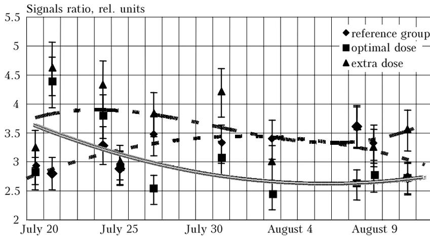
**Fig. 2.** Ratio of fluorescence signals at 685 and 740-nm wavelengths for birch transplants at different concentrations of easily hydrolyzable nitrogen added to soil.
