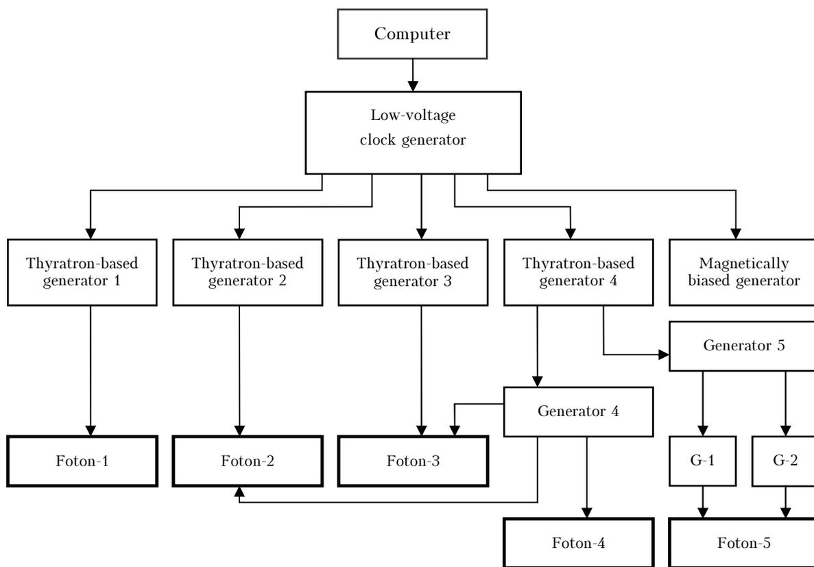
Fig. 2. Block-diagram of the clock and startup system.
