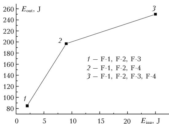
Fig. 3. The output energy of Foton-5 under a double-pass amplification versus the strength of the input signal.
