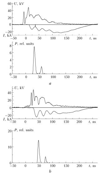
**Fig. 3.** Oscillograms of the voltage pulses at the discharge gap, discharge current, and laser pulse: the mixture is  $N_2/NF_3 = 75/3$  Torr;  $C_p = 10$  nF;  $C_0 = 70$  nF;  $C_1 = 2.45$  nF;  $U_p = 27$  kV;  $U_0 = 35$  kV; (*a*) is the laser with the capacitive energy storage; (*b*) is the laser with the inductive energy storage.
