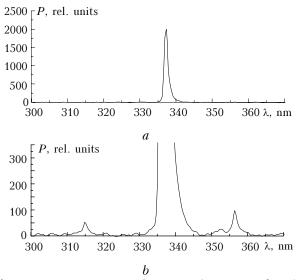
**Fig. 4.** Emission spectrum of nitrogen laser pumped with the generator with an inductive energy storage: the mixture is  $N_2/NF_3 = 75/3$  Torr,  $U_0 = 35$  kV,  $U_p = 25$  kV,  $C_p = 10$  nF, (*a*) attenuated by 250 times; (*b*) with the attenuation by 50 times.
