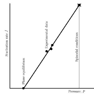
**Fig. 5.** Scheme of algorithm for the computer semi-empirical construction of nucleation rate surfaces.
