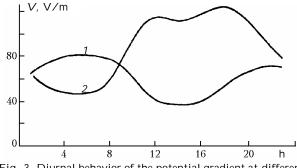
Fig. 3. Diurnal behavior of the potential gradient at different distances from Baikal'sk: 5 (1) and 20 km (2).
