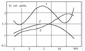
Fig. 1. Variation of the potential gradient with distance: BPPP-water area (1); Murino-water area (2); Tankhoi-water area (3).
