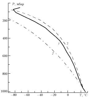
**Fig. 2.** *PT*-curves for the atmosphere above the ocean surface: measured in the equatorial zone (1), calculated for the ascending trial volume of dry air (2), calculated for the ascending trial volume of air with the relative humidity of 85% at the level of 10 m above the surface (3). Air temperature near the ocean surface is  $27^{\circ}$ C.
