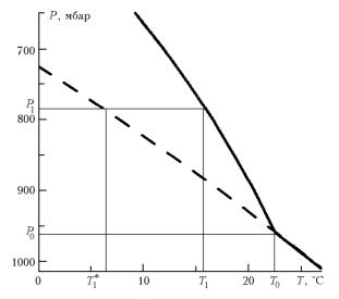
**Fig. 1.** Temperature conditions of trial air volume rising from the ocean surface; air temperature near surface is  $27^{\circ}$ C, relative humidity is 85%; dry adiabat (dashed line), adiabatic expansion of humid air (solid curve);  $P_0$  is the height (in units of pressure), at which water vapor begins to condense.
