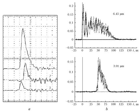
**Fig. 2.** Time dependence of lasing (in rel. units): total pulse (a):  $\lambda \sim 1$ , 3, 6.45 (1), 3 (2), and 1 µm (3); lasing pulses at the lines  $\lambda = 6.45$  and 3.01 µm (b); the scale graduation of the oscilloscope is 50 ns.
