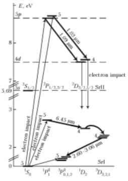
**Fig. 3.** Partial scheme of the energy levels of the SrI atom and SrII ion: the dashed lines are for convergence limits of the series of one-electron and two-electron excitation of the strontium atom.
