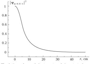
**Fig. 3.** Dependence of the intensity of the principal mode (m = 0, N = 1) on *r*.
