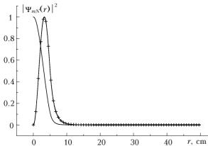
**Fig. 2.** Dependences of the normalized mode intensities  $|\Psi_{m=1, N=1}|^2$  on the radius with m = 0, N = 1 (solid curve) and m = 1, N = 1 (curve marked by +).
