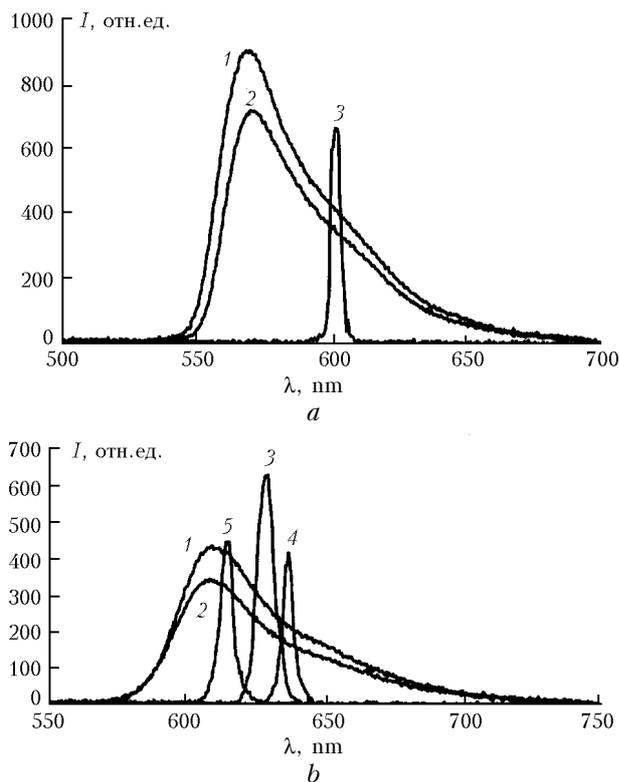
**Fig. 3.** Emission spectra of Rhodamine 6G (*a*) and phenalemine-512 (*b*) in ethanol (1–4) and PMMA (5): laser-induced fluorescence (1), TPLu (2), lasing (3–5).
