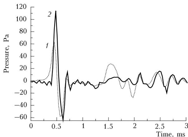
**Fig. 3.** The result of numerical reconstruction of acoustic response of the plasma source:  $d = 141$  m;  $T = 288$  K;  $RH = 75\%$ . With the compensation of only spherical divergence (dashed line) (1); total compensation including the reflection noise (solid curve) (2).
