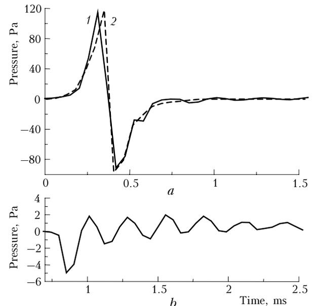
**Fig. 1.** An acoustic response of the quasispherical plasma source.  $d = 16$  cm,  $T = 291$  K,  $RH = 78\%$ , experiment (1); model (2); the pulsations of a plasma source (b) (10 times magnification as compared to a).
