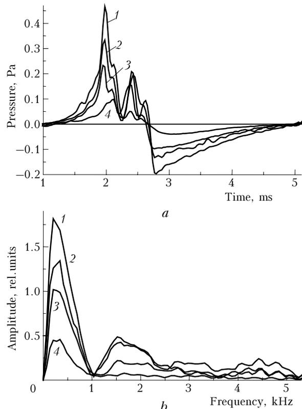
**Fig. 5.** The result of reconstruction of acoustic pulses generated by the HPLR channel and recorded by acoustic receiver at 30-m distance (a), and their frequency spectra (b) for different values of the laser power density: 1.7 (1); 1.36 (2); 0.87 (3);  $0.29 \text{ J/cm}^2$  (4);  $d = 30$  m,  $T = 291$  K,  $RH = 71\%$ .
