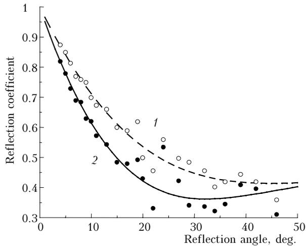
**Fig. 2.** The reflection coefficient of acoustic responses of the plasma source by the underlying surface based on the sound pressure: dry soil (1); the same region after rain (2). Field measurements are denoted by the points, theoretical approximation is denoted by the lines.
