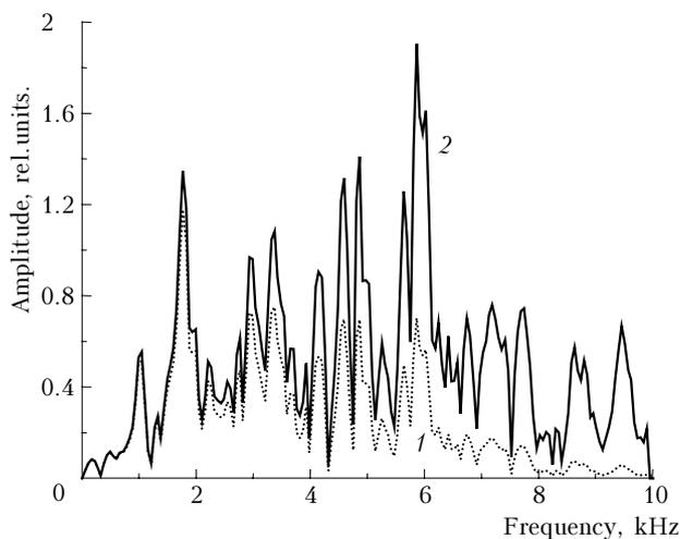
**Fig. 4.** The numerically reconstructed frequency spectrum of acoustic characteristics of the cluster of the plasma cells.  $d = 160$  m,  $T = 288$  K;  $RH = 75\%$ ; without the account of the frequency transformation of acoustic responses (1); with account for such responses (2).
