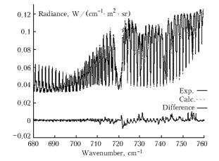
Fig. 10. Fitting of the IMG spectrum and spectrum simulated based on the retrieved temperature profile (see Fig. 8).
