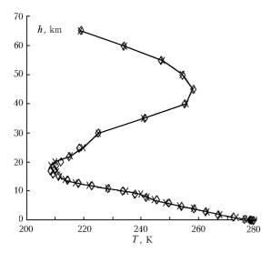
Fig. 1. Vertical temperature profile and its expansions (3) with the number of terms equal to 10 (rhombs) and 20 (crosses).
