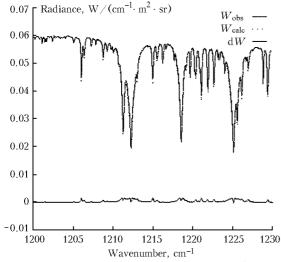
**Fig. 5.** Fitting of the initial model spectrum and spectrum simulated based on the retrieved profile of water vapor concentration (see Fig. 3).
