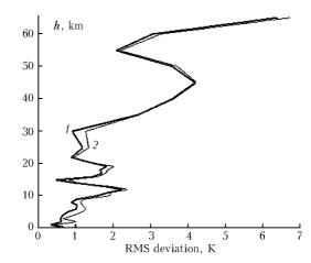
**Fig. 6.** RMS error of retrieval of the vertical temperature profile from model spectra neglecting noise (curve *1*) and with the ADEOS /IMG noise level (curve *2*).
