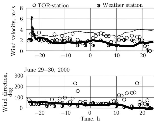
**Fig. 6.** Comparison of calculated and measured wind velocity and direction in Tomsk on June 29–30 of 2000. The designations are the same as in Fig. 4.
