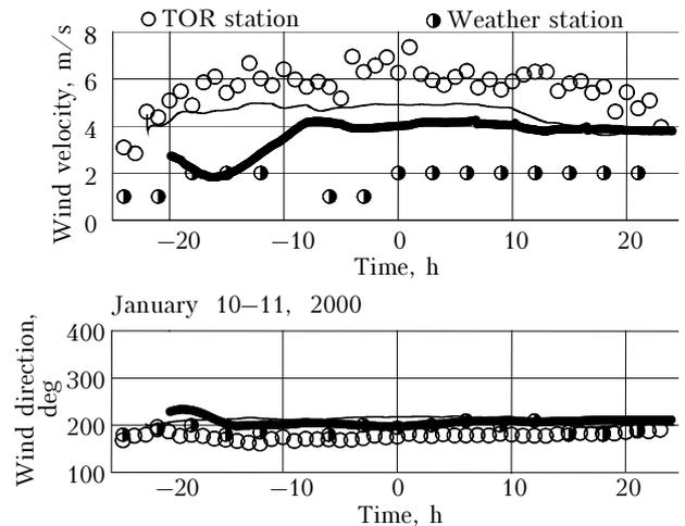
**Fig. 4.** Comparison of calculated and measured wind speed and direction in Tomsk on January 10–11 of 2000: data of the weather stations (half-open circles), observations at the TOR station (open circles), one-dimensional model (1)–(7) (thick solid curve), calculation by 3D mesoscale non-hydrostatic model (thin curve). Negative values on abscissa correspond to the first day of the chosen period, and positive values correspond to the second day.
