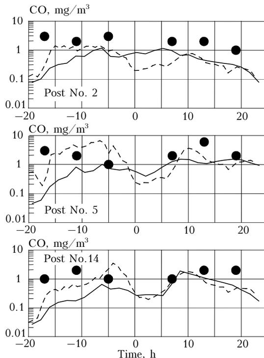
**Fig. 8.** Variation of the CO concentration at ecological posts in Tomsk on September 7–8 of 2000: observations (circles), calculation based on 1D empiric model (dashed curve), calculation using 3D prognostic mesoscale model (solid curve).
