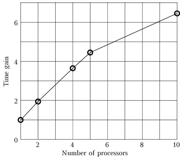
**Fig. 3.** Time gain of the parallel computational process vs. the number of processors involved.
