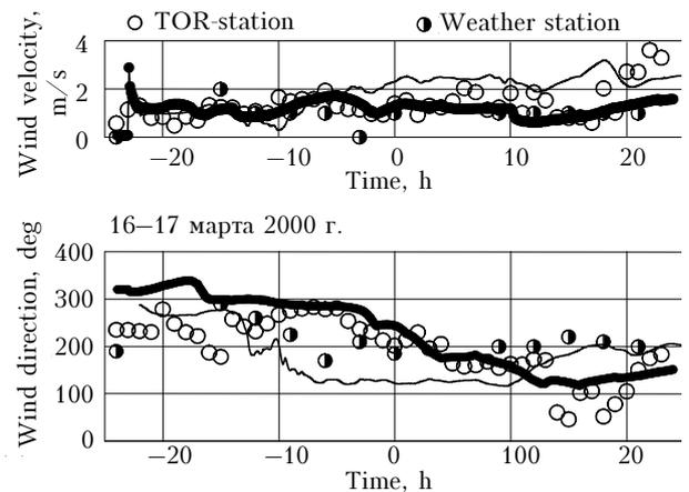
**Fig. 5.** Comparison of calculated and measured wind velocity and direction in Tomsk on March 16–17 of 2000. The designations are the same as in Fig. 4.
