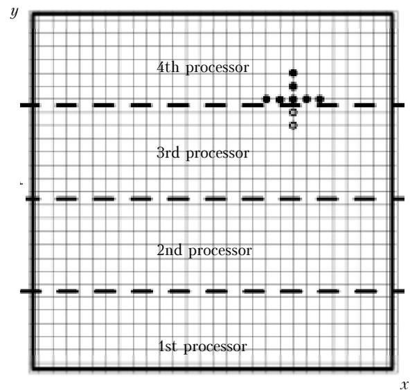
**Fig. 1.** Computational grid in the plane  $xOy$  with indicated distribution of regions over four processors. The difference mask is shown on the near-boundary grid line. Open circles indicate the grid values to be received from the neighboring processor.
