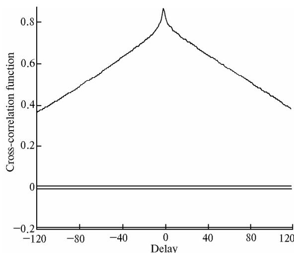
Fig. 2. Cross-correlation function of CO and NO concentration.
