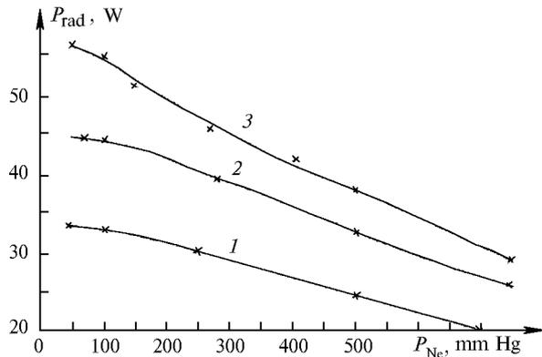
Fig. 8. Dependence of the total mean output power of Crystal LT-30 Cu AE (1), Crystal LT-40 Cu (2), and Crystal LT-50 Cu (3) on neon pressure at power consumed from the rectifier  $P_{rect} = 3.2, 4.0, \text{ and } 5.5$  kW and pulse repetition frequency  $f = 10$  kHz.
