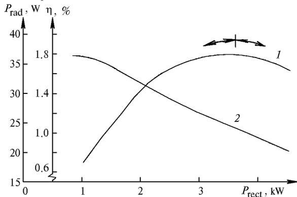
**Fig. 5.** Instantaneous values of the output power (1) and efficiency (2) vs. power consumed from rectifier with the voltage doubling scheme at  $T_{\text{ch}} = 1630^\circ\text{C}$  for Crystal LT-30 Cu gas-discharge tube.
