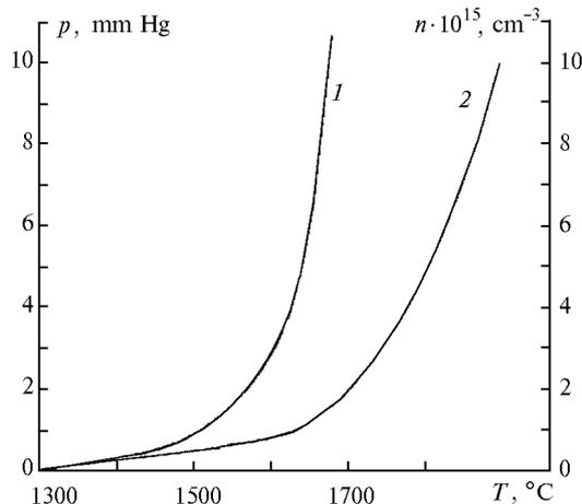
Fig. 3. Temperature dependence of the partial pressure (1) and concentration of copper atoms (2).
