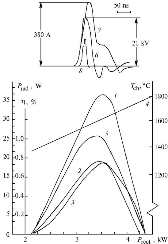
**Fig. 4.** Total mean output power (1), power at separate wavelengths: 0.51 (2) and 0.58  $\mu\text{m}$  (3), temperature of the discharge channel (4), efficiency (5) vs. power from rectifier with voltage doubling scheme for Crystal LT-30 Cu. Oscillograms of voltage (6), discharge current (7), and radiation pulses (8) of AE.
