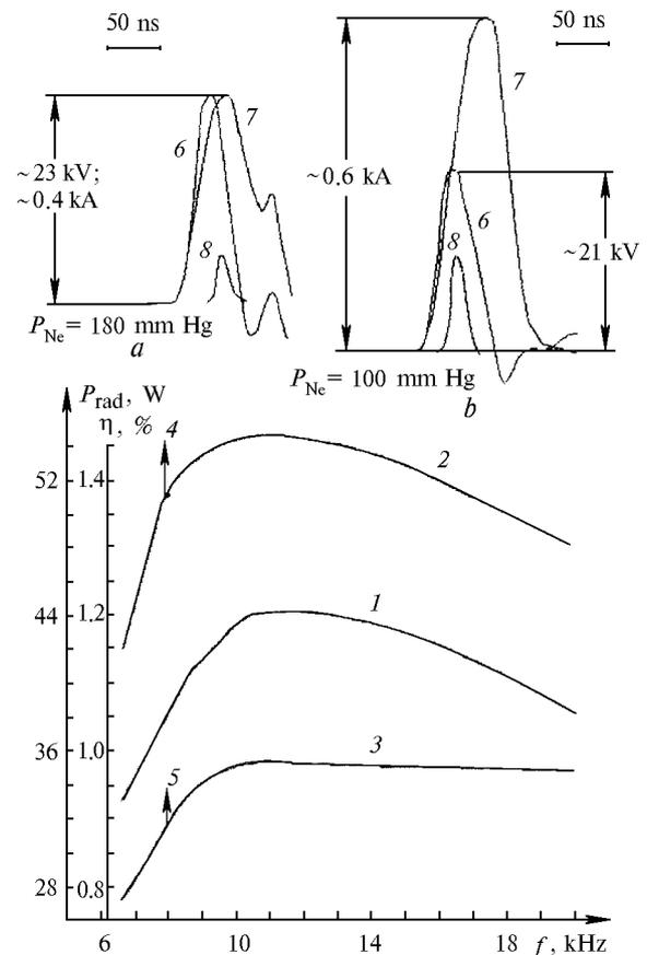
Fig. 9. Dependence of the total mean output power for Crystal LT-40 AE (1) and Crystal LT-50 Cu AE (2) and efficiency (3) on the pulse repetition frequency. Oscillograms of voltage (6), discharge current (7), and radiation pulses (8) for Crystal LT-40 Cu AE (a) and Crystal LT-50 Cu AE (b) at a pulse repetition frequency  $f = 10.5$  kHz.
