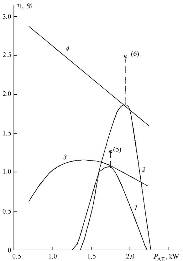
**Fig. 7.** Dependence of the efficiency in a stable thermal (1, 2) and transient (instantaneous) (3, 4) regimes on power deposited into the AE with the traditional excitation scheme (1, 3) and voltage doubling scheme (2, 4) for Crystal LT-30 Cu gas-discharge tube.
