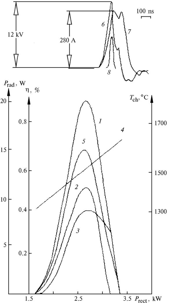
Fig. 2. Total mean output power (1), power at  $\lambda = 0.51$  (2) and  $0.58 \mu\text{m}$  (3), temperature of AE discharge channel (4), and efficiency (5) vs. power from the rectifier with the traditional scheme for a Crystal LT-30 Cu active element.
