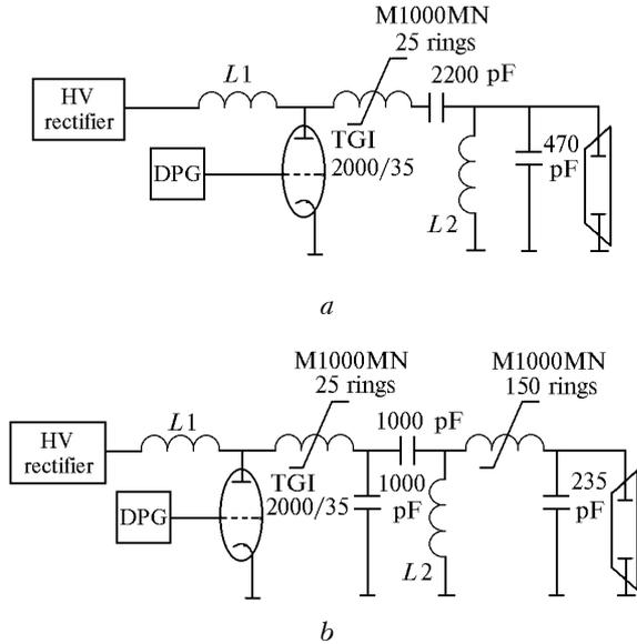
Fig. 1. Electric circuits of a pulsed power supply.
