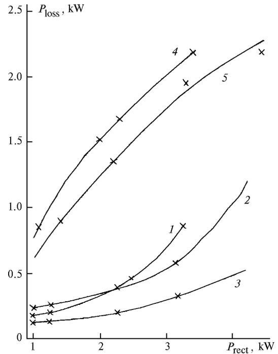
**Fig. 6.** Dependence of power loss in a thyatron with thyatron (1, 2), magnetic compression unit (3), and AE (4, 5) on power consumed from rectifier in the case of the traditional excitation scheme (1, 4) and voltage doubling scheme (2, 3, 5) for Crystal LT-30 Cu gas-discharge tube.
