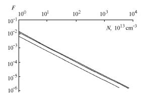
Fig. 3. Radiation trapping factor vs. concentration of thulium atoms for transitions with the wavelengths of 388.313, 374.407, and 371.792 nm.
