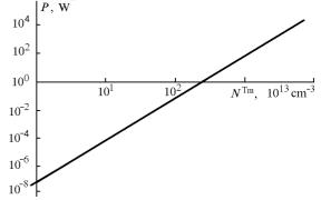
Fig. 4. Output power vs. concentration of thulium atoms.
