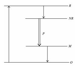
**Fig. 2.** Generalized scheme of the lasing levels of self-limited transitions with indirect excitation of the upper lasing levels: resonance level (R); nonresonance (upper lasing) level (NR); metastable (lower lasing) level (M); ground state (O); the lasing transition (P).
