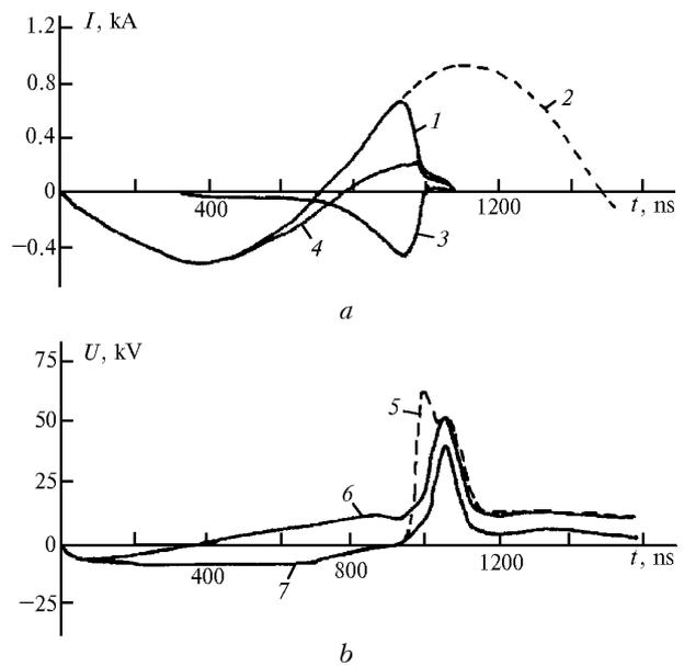
**Fig. 4.** Oscillograms of current and voltage at idle operation of the setup ( $C_1 = 16.5\ \text{nF}$ ,  $C_2 = 0$ ):  $I_2$  (1),  $I_2$  at the short-circuit opening switch (2),  $I_3$  (3),  $I_4$  (4),  $U_1$  (5),  $U_3$  (6), and  $U_2$  (7).
