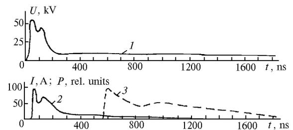
**Fig. 10.** Oscillograms of voltage across gas-discharge gap (1), discharge current (2), and CO<sub>2</sub> laser pulse (3) (CO<sub>2</sub>:N<sub>2</sub>:He = 1:3:3,  $C_1 = 16.5$  nF, tube length is 400 mm,  $d = 9.5$  mm,  $p = 27$  Torr).
