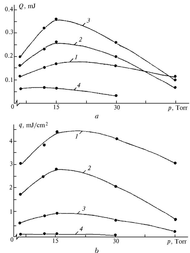
Fig. 7. Output energy (a) and output energy density (b) of nitrogen laser vs. nitrogen pressure in discharge tubes of different diameter  $d = 2.2$  (1), 3.4 (2), 6.8 (3), and 9.5 mm (4) (tube length of 200 mm,  $C_2 = 330$  pF).
