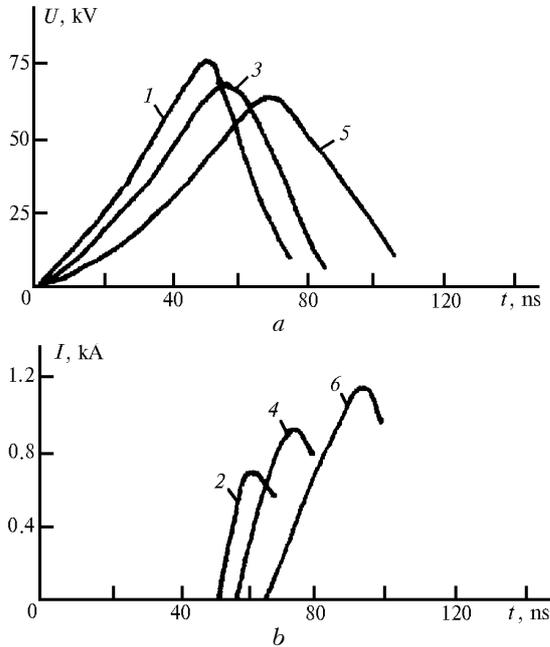
**Fig. 5.** Oscillograms of voltage across a gas-discharge tube (1, 3 – 5) and the discharge current (2, 4, 6). Discharge in nitrogen,  $p = 30$  Torr,  $C_2 = 94$  (1, 2), 170 (3, 4), and 330 pF (5, 6).
