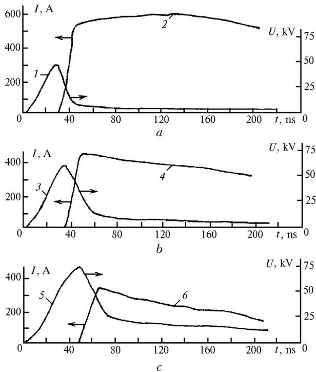
**Fig. 6.** Oscillograms of the discharge current (1, 3 – 5) and voltage across a gas-discharge tube (2, 4, 6). Discharge in nitrogen,  $C_2 = 0$ ,  $p = 6$  (a), 15 (b), and 30 Torr (c).
