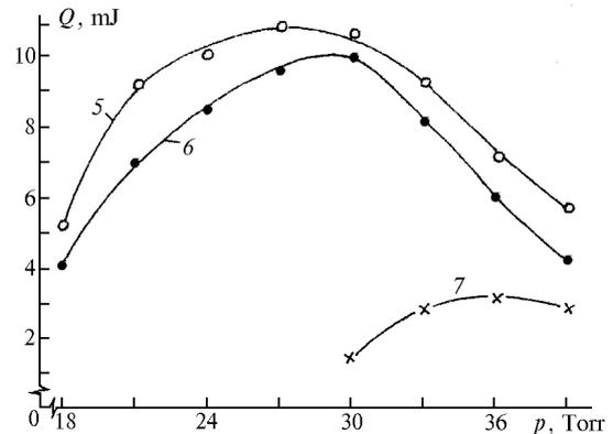
**Fig. 9.** Output energy of CO<sub>2</sub> laser vs. pressure of the working mixture CO<sub>2</sub>:N<sub>2</sub>:He = 1:3:3; the tube is 400 mm long:  $d = 9.5$  mm,  $C_1 = 16.5$  nF,  $C_2 = 0$  (1);  $d = 9.5$  mm,  $C_1 = 16.5$  nF,  $C_2 = 170$  pF (2);  $d = 6.8$  mm,  $C_1 = 4.4$  nF,  $C_2 = 0$  (3).
