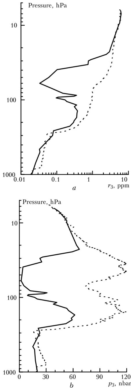
**Fig. 5.** The VOD profiles at the stations Syova (69°S, 40°E) on 22 September 1998 (solid curve) and Yakutsk (62°N, 130°E) on 19 March 1995 (dashed curve); (a) the values are given in the units of the mixing ratio (ppm); (b) in the units of partial pressure (nbar).
