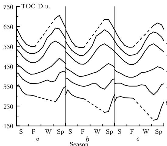
**Fig. 4.** The annual mean variation of zonal mean TOC for different latitudinal belts: 80–70°N (1); 70–60°N (2); 60–50°N (3); 50–60°S (4); 60–70°S (5) and 70–80°S (6) (for lower curve the numerical values plotted on the ordinate correspond to reality; each subsequent curve is elevated by about 50 D.u.), during different observation periods: (a) December 1978–November 1982; (b) December 1990–November 1994; (c) August 1996–July 1999.
