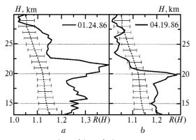
FIG. 2. Vertical profiles of the scattering ratio with the pronounced volcanic aerosol layers measured on January 24, 1986 (Fig. 2a) and April 12, 1986 (Fig. 2b). The average profile of the scattering ratio, calculated for the background stratospheric state, is also shown by the dashed curve.
