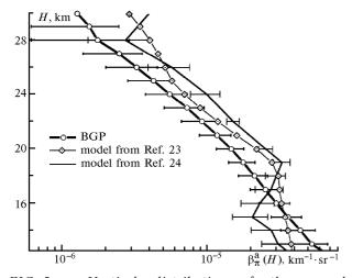
FIG. 5. Vertical distribution of the aerosol backscattering coefficients at  $\lambda = 532$  nm, obtained by averaging of the individual experimental profiles of  $\sum \beta_{\pi}^{a}$  measured under background conditions in 1989– 1990, in comparison with the aerosol models.
