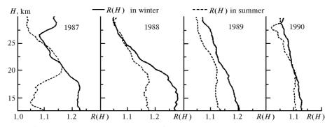
FIG. 3. Vertical winter (the solid curves) and summer (the dashed curves) profiles of the scattering ratio at  $\lambda = 532$  nm for the indicated years.
