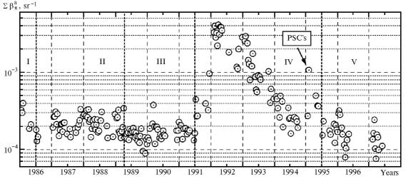
FIG. 1. Temporal behavior of the total aerosol backscattering coefficient  $\sum \beta_{\pi}^{a}$  at  $\lambda = 532$  nm between 15–30 km over Tomsk (56.5°N, 85.0°E).
